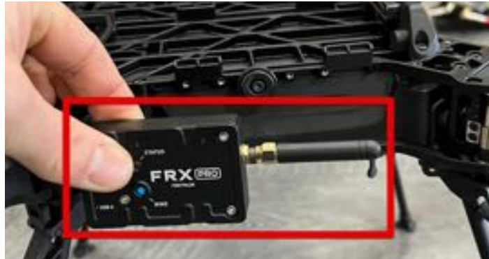
Figure 1. Example of an unacceptable radio mounting location that has direct line between antenna and the plastic tub on side of chassis
