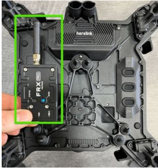
Figure 3. Example of improved radio mounting location under the Astro chassis
