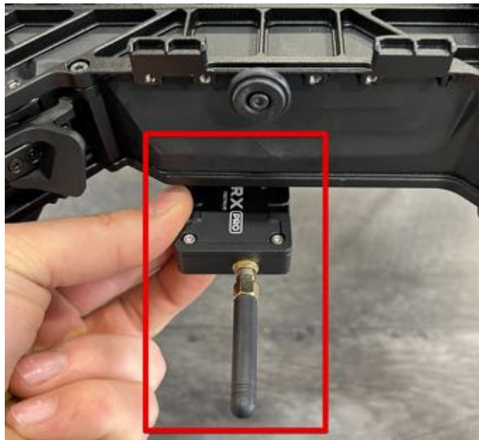
Figure 2. Example of another unacceptable radio mounting location
