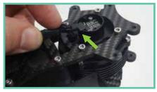
30. Plug both motor wires back in, being careful not to force them as they are keyed to go in one way.
