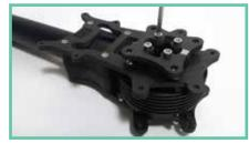
25. Reinstall the carbon plate to the motor, line up your marks and reuse the original hardware with thread lock.
