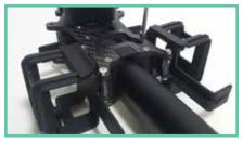
28. Ensure both cages are installed tight with the doors facing up, and your pan tube is seated fully and the spine is facing down.
