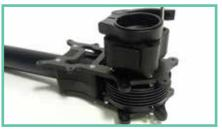
26. (optional) Install your Toad in the Hole Quick Release with the lever facing towards the front.
