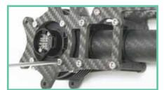
18. Remove the 8 bolts with a 2.5mm driver, and the 5 button head bolts with a 2mm driver. Use pliers to hold the posts if they spin.
