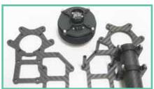
19. Pull the carbon plates apart, save the motor and set aside or discard the rest.
