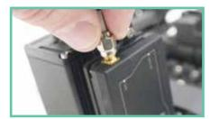
07. Unscrew the GPS SMA connector.
