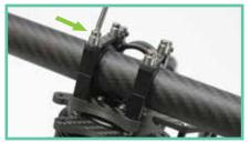
01. Loosen the 4 bolts holding the handle bar on to the pan assembly of your MoVI M10.
