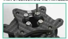
16. Remove the 4 bolts from the motor and set the carbon plate and bolts aside.
