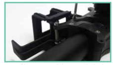
27. Install battery cages with the M3X8 socket head bolts - orient with the lever of the door facing up.
