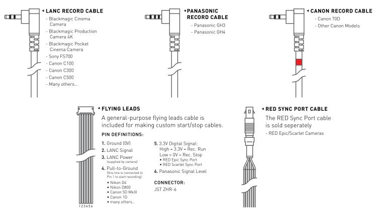
NOTE: This is not a complete list of all compatible camera models that work with each of the cables. Test the cables to identify which cable goes to your camera. The 5-pin ZH to 3-pin ZH Record Cable that is included in the kit will be for future use. Do not throw it away.
