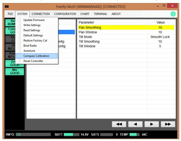
Both the MōVI and MIMIC require compass calibrations in order for Compass Heading Assist to function properly. To perform a compass calibration on either the MōVI or MIMIC, use the MōVI App. For the MōVI, select System menu, then Compass Calibration and open the terminal to follow the text instructions. For the MIMIC, select the Start Compass Cal setting under the General menu, and click the right arrow to initiate it. Open the terminal and follow the text instructions.
