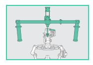
07. Once alignment is set, fully tighten levers on the Handle Clamp. Insert the Handle Clamp via the Toad (Male Adapter on the Handle Clamp) into the TITH (Female Adapter).
