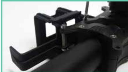
27. Install battery cages with the M3X8 socket head bolts - orient with the lever of the door facing up.
