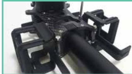
28. Ensure both cages are installed tight with the doors facing up, and your pan tube is seated fully and the spine is facing down.
