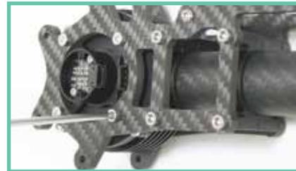
18. Remove the 8 bolts with a 2.5mm driver, and the 5 button head bolts with a 2mm driver. Use pliers to hold the posts if they spin.
