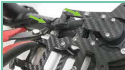
03. Lay unit on its side, cut and remove zip ties from pan motor assembly.
