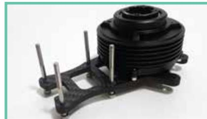
21. Insert the 4 M3X37 screws provided through the carbon plate with motor as shown, and lay flat on your work surface.
