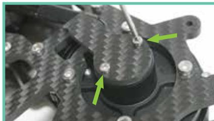
04. Remove these screws, the carbon plate, and metal plate underneath.
