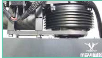
11. Install your new keyed pan assembly as shown, the levers should be pointing to the left of the unit.
