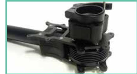
26. (optional) Install your Toad in the Hole Quick Release with the lever facing towards the front.
