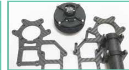
19. Pull the carbon plates apart, save the motor and set aside or discard the rest.
