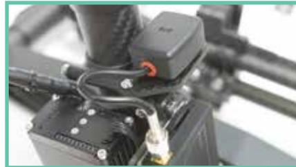
16. Install your GPS back onto the plate as shown and screw back on the SMA connector.
