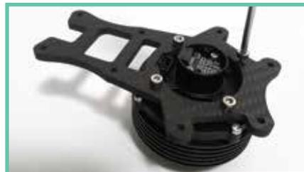
21. Using the carbon plate without threaded inserts, install it to the motor as shown so the plug fits in the cut out of the carbon and attach with your original socket head bolts.
