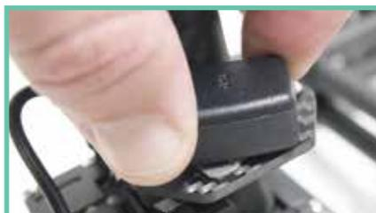
08. Twist the GPS module off of the carbon plate and clean any tape from GPS, set aside.
