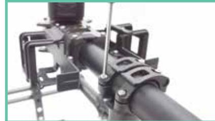
29. Slide the pan assembly on to the vertical tube - you may need to loosen the clamp slightly to get it started. Tighten these screws and adjust clamps to desired snugness.
