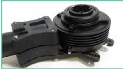
23. Place the metal tube with plastic clamps over the 4 bolts as shown; making sure the keyed rib is on the same side as the plugs on the motor.
