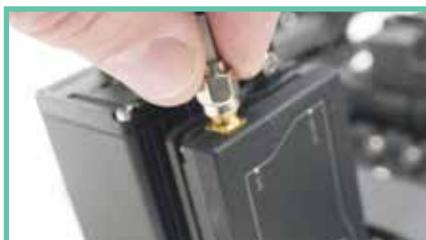
07. Unscrew the GPS SMA connector.
