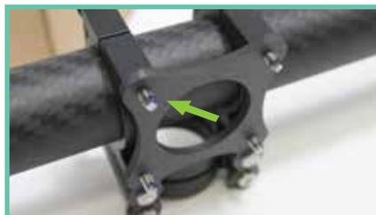
(optional) Loctite screws and Install Toad in the Hole Male.
