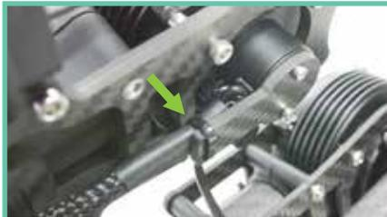
31. Reinstall metal and carbon cover, use a zip tie to securely tighten the wires to the carbon plate around shrink tubing on wire.
