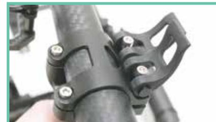
06. Loosen pan adjustment levers, or unscrew pan clamp and remove pan assembly from unit and set aside.
