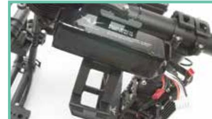
33. Place a Freely M10 Aux Pack into the battery holder and close. Plug in battery.
