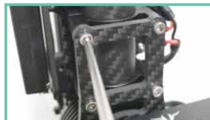
09. Loosen the 4 screws holding the vertical tube approx 2-5 turns until the tube is just loose enough to turn.
