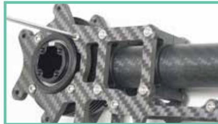
17. Remove the 4 button head bolts with a 2mm driver; use caution and make sure the driver is fully seated to avoid stripping.
