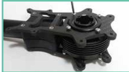
24. Place the carbon with inserts over the motor, and install the 4 button head screws into the motor. Make sure the threaded inserts are facing out.
