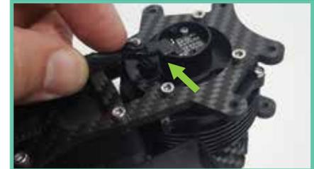
30. Plug both motor wires back in, being careful not to force them as they are keyed to go in one way.
