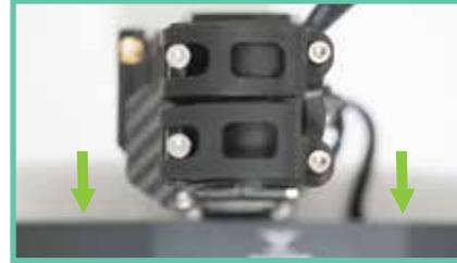
13. From above, look down at the gimbal and twist the keyed quick release until it is as square as possible with the roll beam. (this can be adjusted later.)
